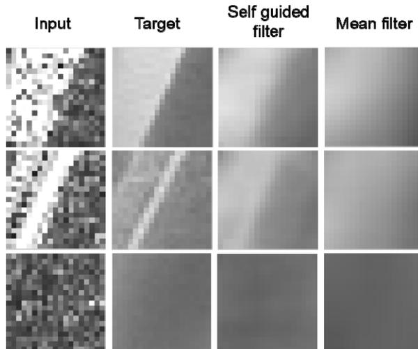
Fig. 2. Training dataset examples. The first and second rows are the patches near depth discontinuities. The third row is a patch on uniform depth.
