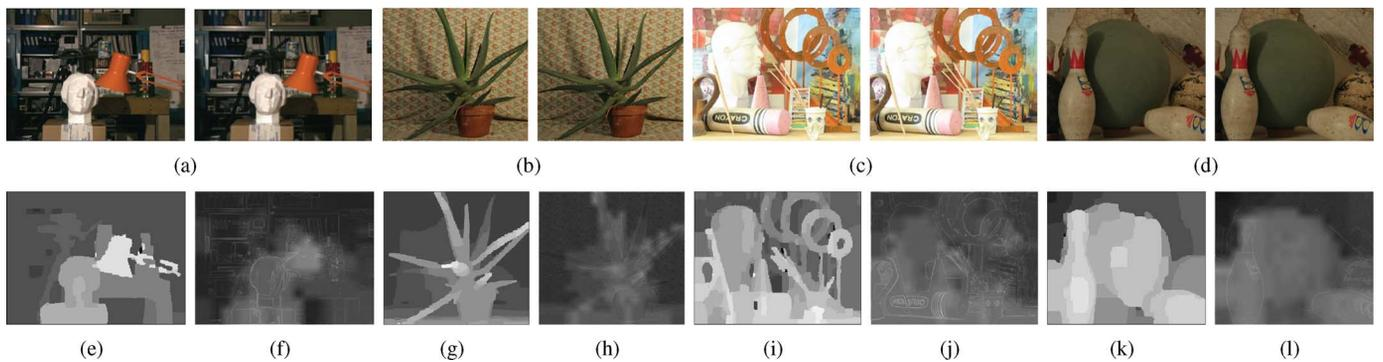
Fig. 2. Input images and the saliency maps. (a)–(d) The Middlebury test images (left and right) [10]. (e), (g), (i), (k) Reference disparity maps using belief propagation (BP) algorithm [11]. (f), (h), (j), (l) Estimated saliency maps.
