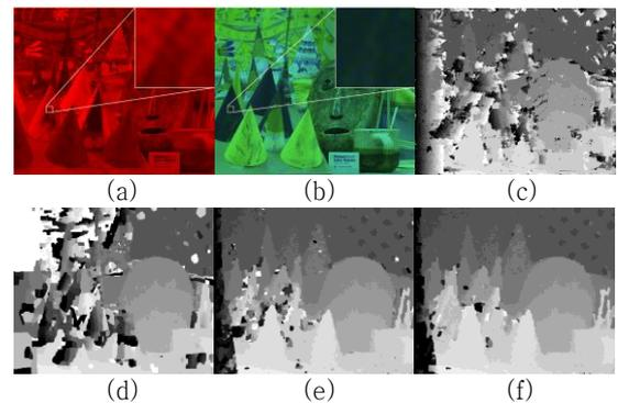
Fig 2. Disparity Results of each data cost (BP = bad pixels percentage). (a) Cones data (left image); (b) Cones data (right image); (c) Results of Lin's method [1] (BP = 34.38%); (d) Results of MI [4] (BP = 47.5%); (e) Results of using ANCC (BP = 12.13%); (f) Results of using the proposed AANCC (BP = 9.06%).
